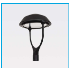
URQ1203060D2 120W Adaptation Urban Street Luminaire 60° 3000K DALI
